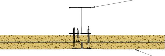
2x12.5mm Knauf Wallboard fixed with SPEEDLINE Drywall Screws at 300mm centres (200mm centres at external angles). Ref to table for fixing length.
